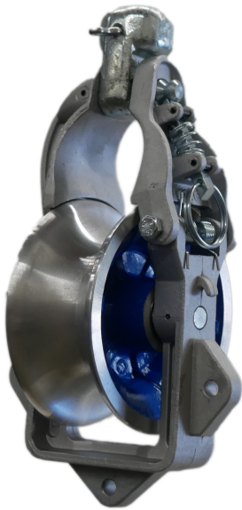
STR-7 Distribution Block 7" O.D, Rim Width 3" Throat Height 3 3/4" Weight 9.3lbs Throat Width 3 1/8" Safe Working Load 2,500lbs
